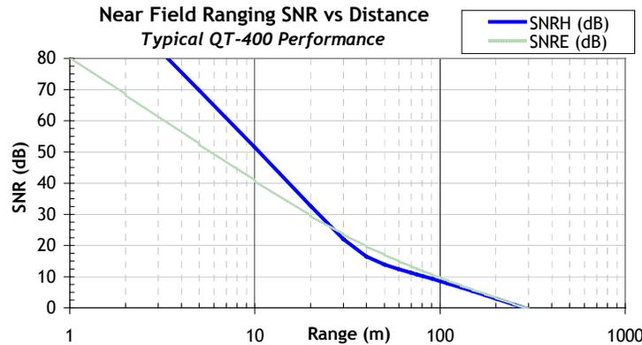
Figure 4: Typical SNR results for Q-Track's QT-400 Starter Kit System. [© 2006, Q-Track].
